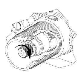
Rotate CW for Cooler (shown)
